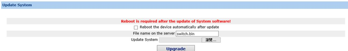
Figure 8: Upgrading the IOS software
