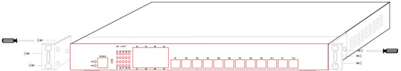
**Figure 2-4** Attach brackets to the Managed Switch.
