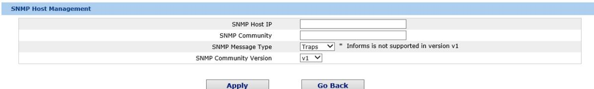
The screenshot shows the 'SNMP Host Management' configuration page. It has a header bar with the title. Below it, there are four input fields: 'SNMP Host IP', 'SNMP Community', 'SNMP Message Type' (with a dropdown menu set to 'Traps' and a note '\* Informs is not supported in version v1'), and 'SNMP Community Version' (with a dropdown menu set to 'v1'). At the bottom, there are two buttons: 'Apply' and 'Go Back'.
