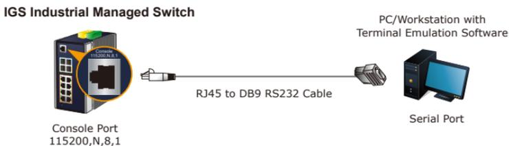
A terminal program is required to make the software connected to the Industrial Managed Switch.
