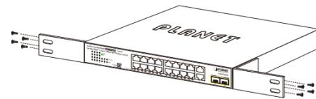
Figure 5-1: Attaching the Brackets to the 802.3at PoE+ Switch.
