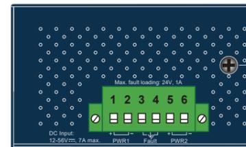
Figure 3: Industrial Gigabit PoE Switch Upper Panel
