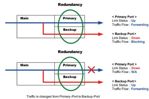
Figure 2: Redundancy Behavior Topology
